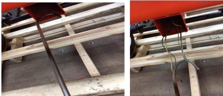
21) Connect ground wire to 16" wire on the main harness and tape the connection. When you pull the wires out the front of the mixer, it should stop at approximately 40-42" from the connector to the frame of the mixer.
