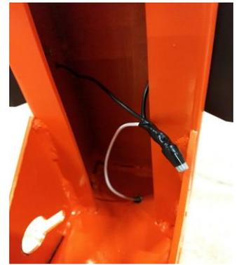
16) Take your small hook and fish wire through the front of the frame, and tape the wire to the frame.
