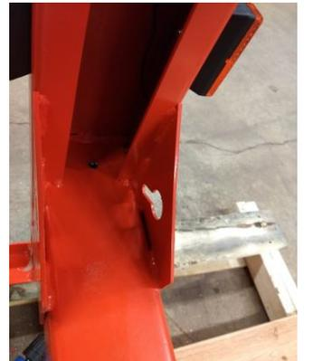
10) 2 feet up, and 1-5/16" in from the base of the mixer (You can make a template with a hole in it for a felt marker) drill a hole for the side marker light.
