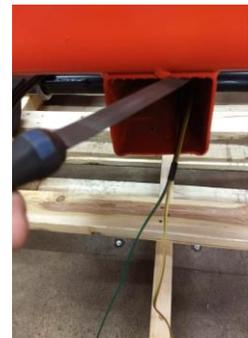
26) Run all wires up and around to the rear of the frame, where the tail lights will be mounted.
