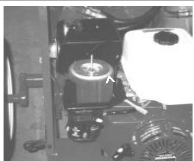
Fig. 25 ENGINE AIR INTAKE FILTER
