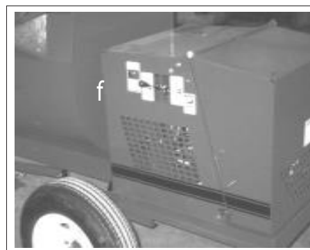
Fig. 3 EMERGENCY STOP SWITCH
